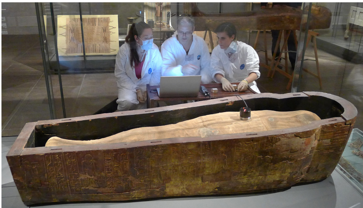
Fig. 1: A phase of a non-invasive water activity (aw) test carried out on the mummy of Kha (Suppl. 8431). Picture by Eurac Research, Institute for Mummy Studies.
