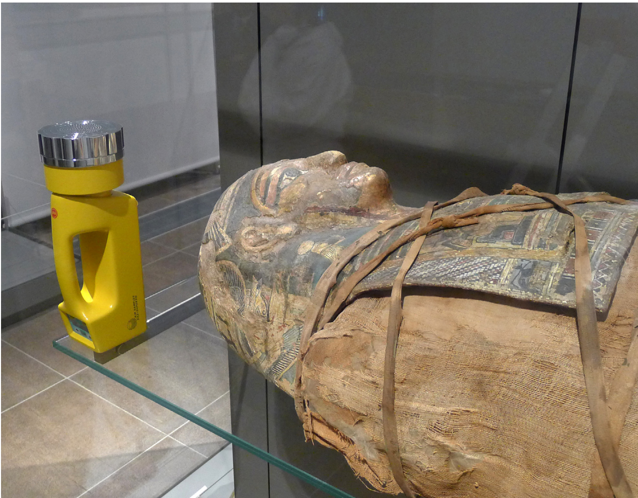
Fig. 4: Sampling of spores present in the air inside display cases (Suppl. 19691). Picture by Marco Samadelli/Eurac Research, Institute for Mummy Studies.
