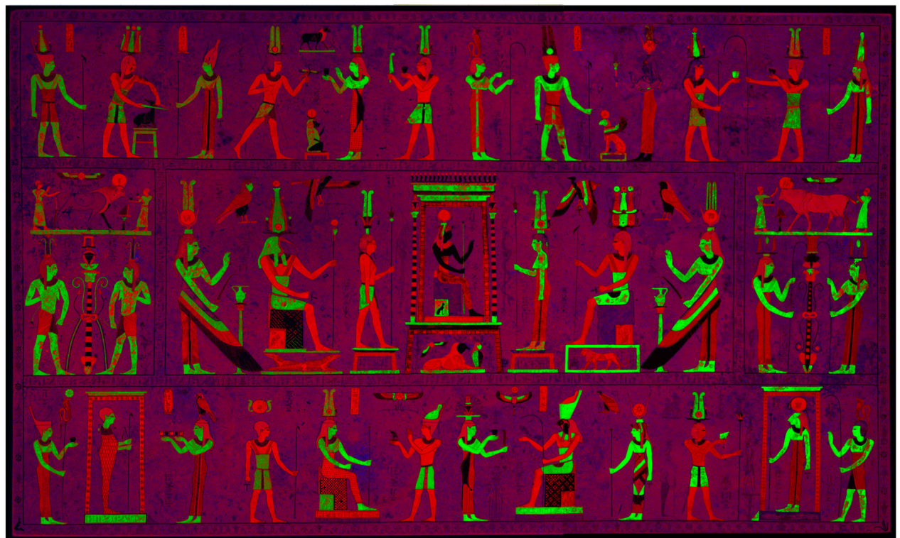
Fig. 9: RGB false color overlay of MA-XRF distribution maps of copper (red channel), tin (blue channel) and zinc (green channel). Where more than one element is present in a single pixel, the resulting color reflects the relative proportion of each element present. Image produced by the authors.
